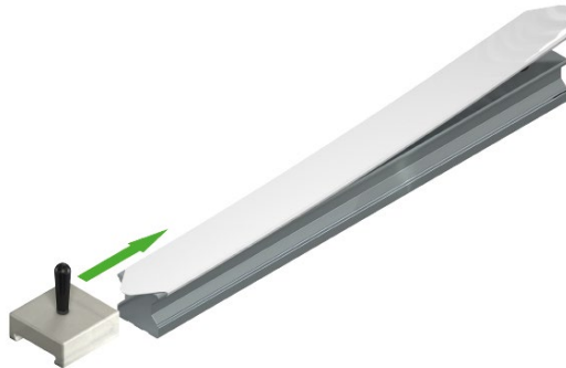
Fig. 4.10: Mounting the cover strip using the assembly tool
